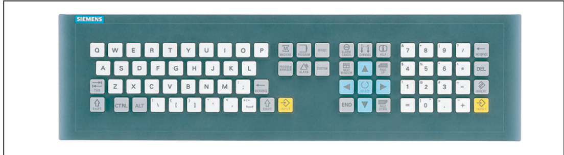
Image 4-1 Layout of CNC full keyboard KB 483C
