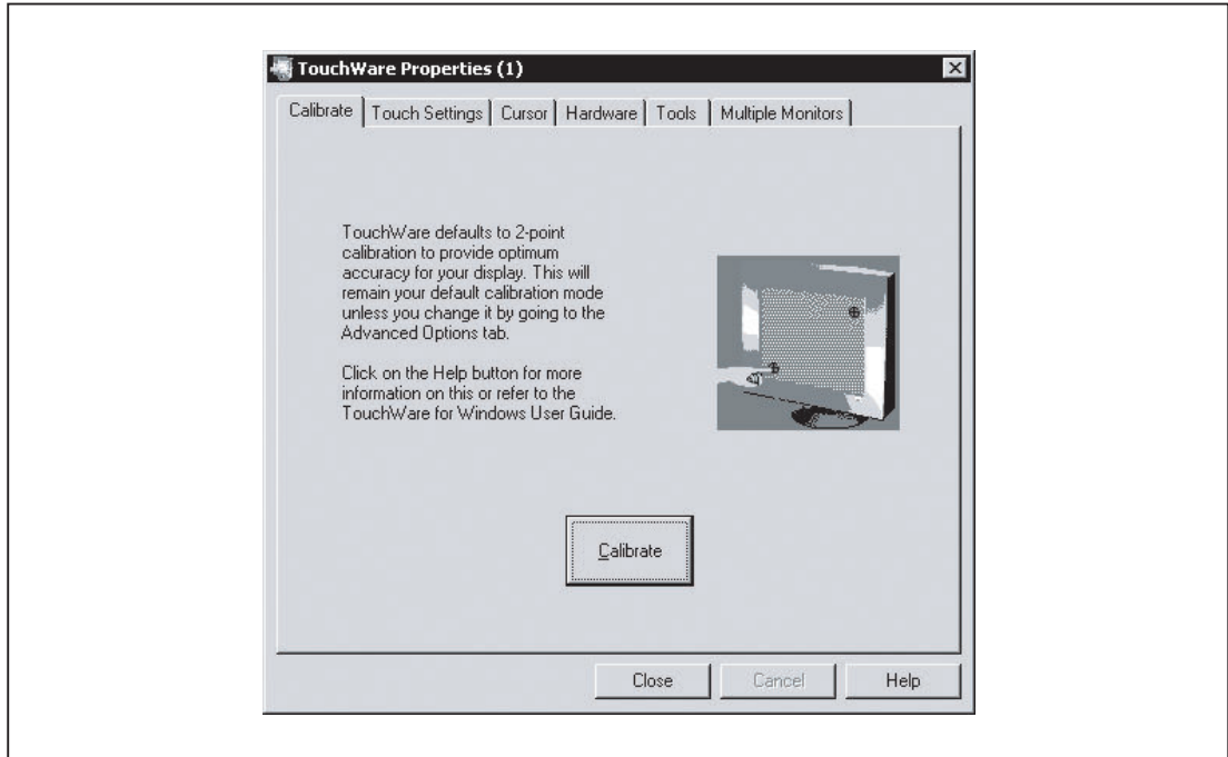
Image 15-20 Menu for touch screen calibration (Touchware version 5.64 SR3)
